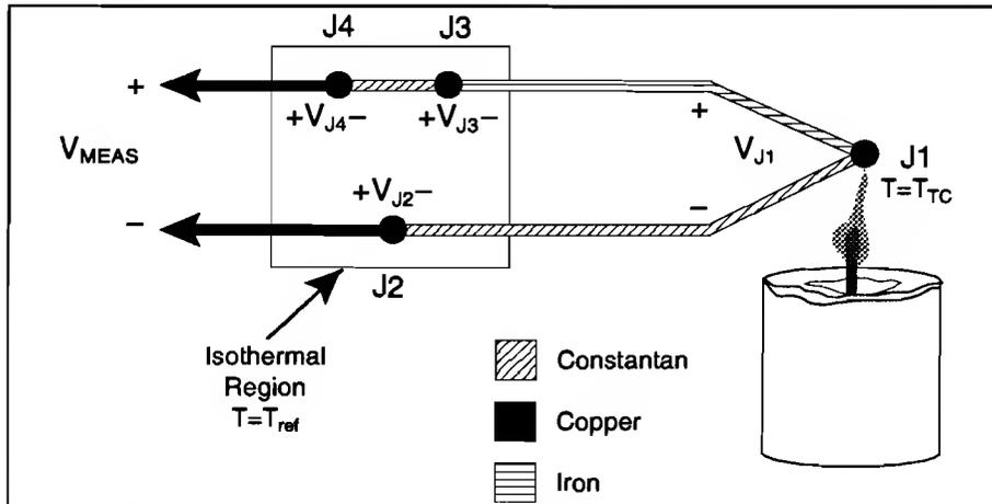
Figure 5. Inserting an Extra Lead in the Isothermal Region
