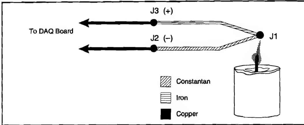
Figure 2. J-Type Thermocouple
