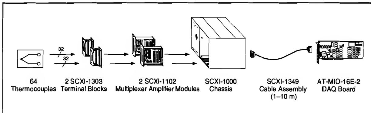
Figure 7. SCXI System for Monitoring 64 Thermocouples
