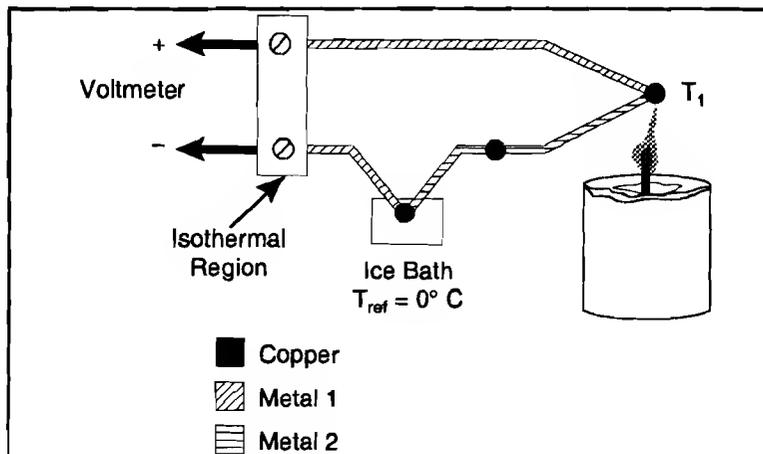
Figure 3. Traditional Temperature Measurement with Reference Junction Held at  $0^\circ\text{C}$
